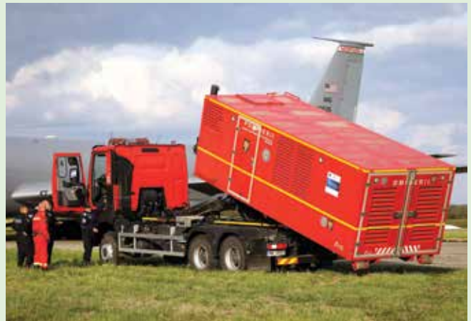
“Type IV - lighting” logistical support container
